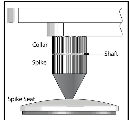
**Method:** Run the textured collar halfway down the threaded shaft away from the spike point. Insert the shaft into the plinth and screw in tight. Now run the collar up to the plinth and lock it finger tight. Repeat for all four spikes.
